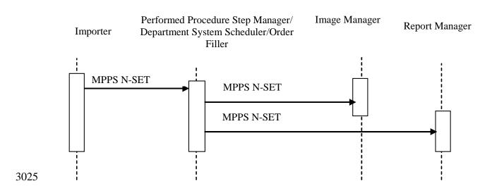
Note: The diagram above shows the sequencing of messages for the Modality Performed Procedure Step SOP Class. Importers will also implement the Storage and Storage Commitment classes. The timing relationship between PPS messages and Storage and Storage Commitment messages is not specified. That is, PPS messages may occur before or after storage requests.
