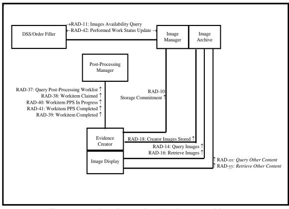
Figure 12.1-1: Post-Processing Workflow Actor Diagram
