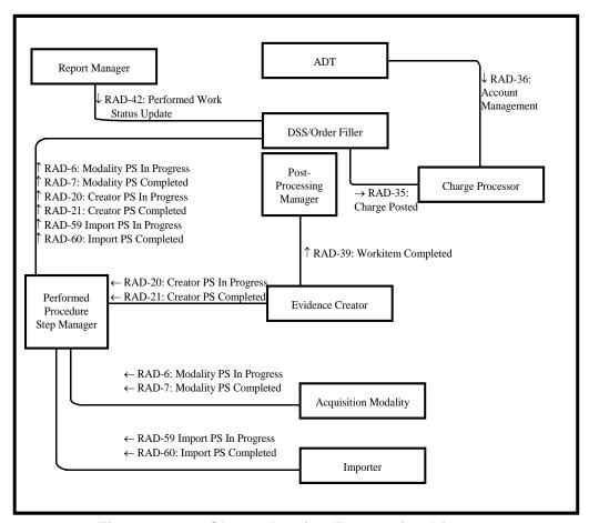
Figure 11.1-1: Charge Posting Transaction Diagram
