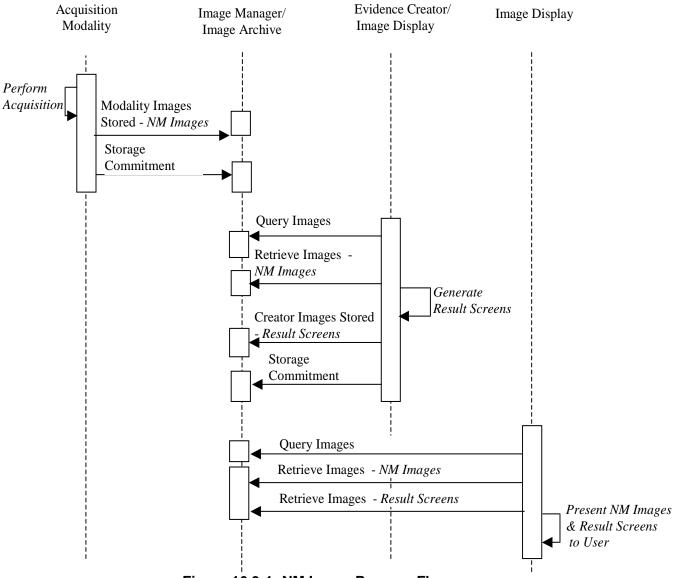
Figure 16.3-1: NM Image Process Flow
