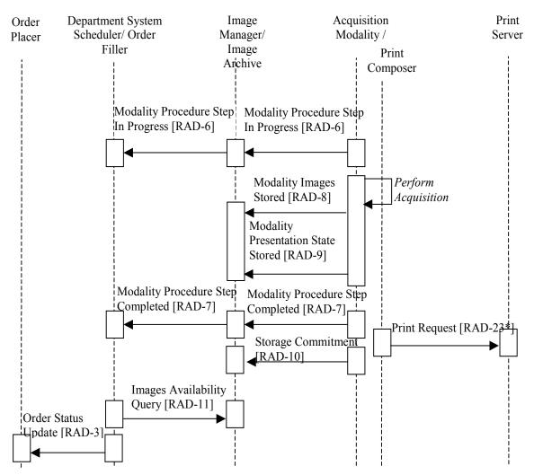
Figure 34.4.2.1-2: Procedure Performance Process Flow in SWF.b.
