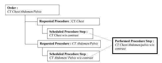
In this example, a single Performed Procedure Step has been performed in response to two Scheduled Procedure Steps. IHE refers to this as a Group Case (see RAD-TF2: 4.6). At the time of reading, the same series of images produced by this Performed Procedure Step would be read once in the context of the CT Chest Requested Procedure and again in the context of the Abdomen/Pelvis Requested Procedure.
