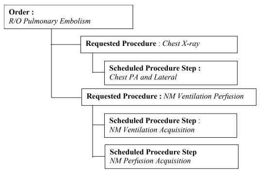
In this Procedure Plan, for this specific Order, two Requested Procedures are defined. The Chest X-ray that will be read and reported by a different radiologist than the NM Ventilation-Perfusion, hence two different Requested Procedures. The NM Ventilation Perfusion Procedure has been scheduled as two different Scheduled Procedure Steps, to account for the fact that the patient will
