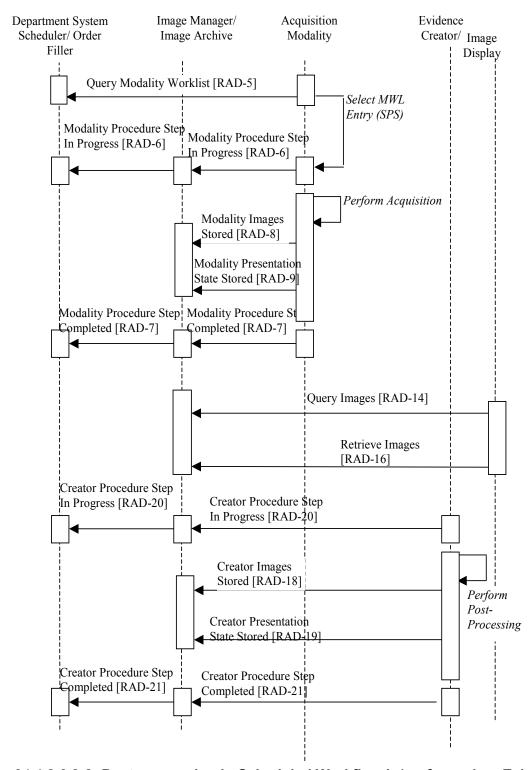
Figure 34.4.2.6.2-2: Post-processing in Scheduled Workflow.b (performed on Evidence Creator)
