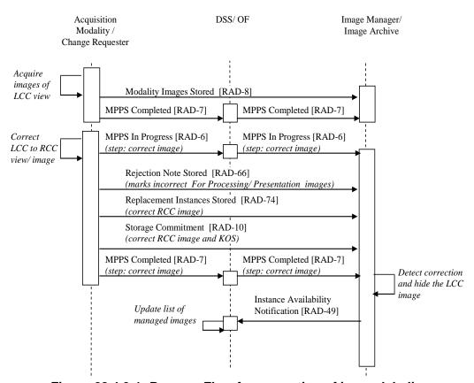
Figure 28.4.3-1: Process Flow for correction of image labeling
