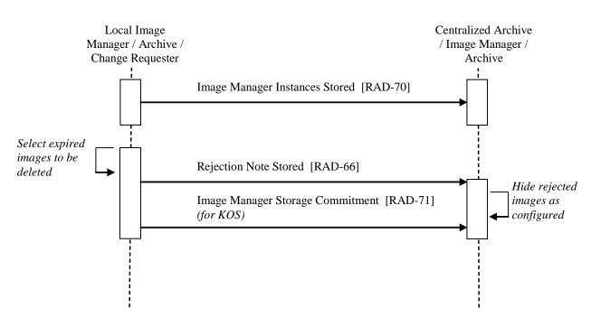
Figure 28.4.1-1. Process Flow for handling expired studies
