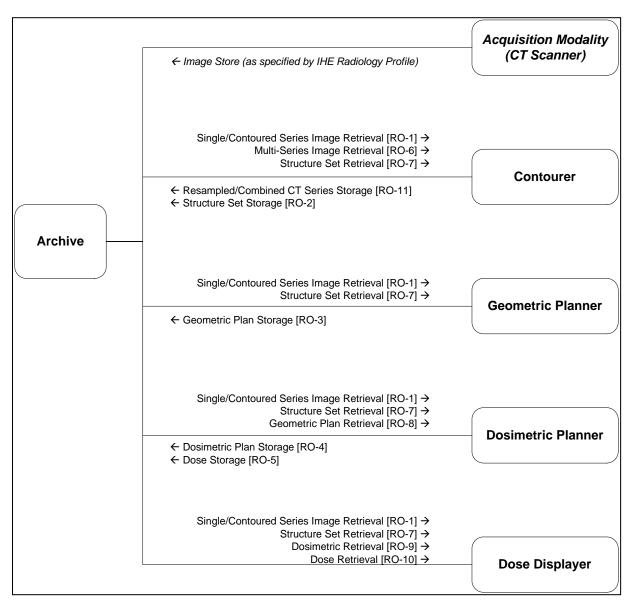
Figure 3.1-1: Basic RT Objects Actor Diagram
