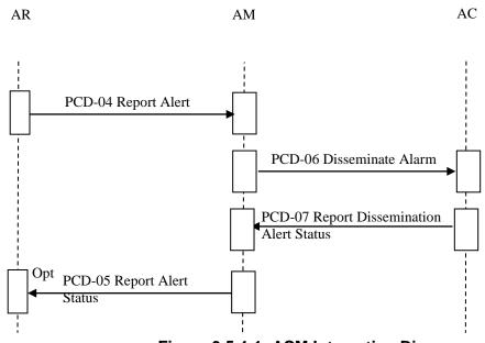
Figure 3.5.4-1: ACM Interaction Diagram
