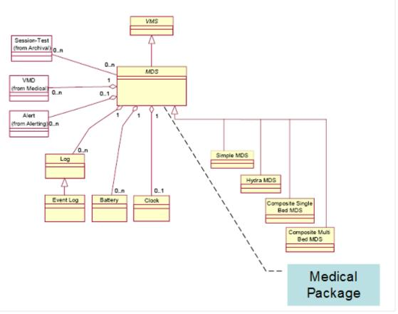
Figure A-1: System Package Model
