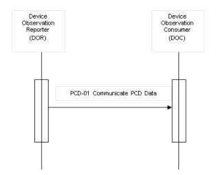
Figure 3.1.4.1-1: Communicate PCD Data Interaction Diagram
