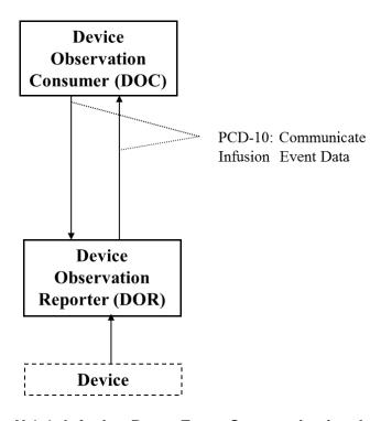
Figure X.1-1: Infusion Pump Event Communication Actor Diagram
