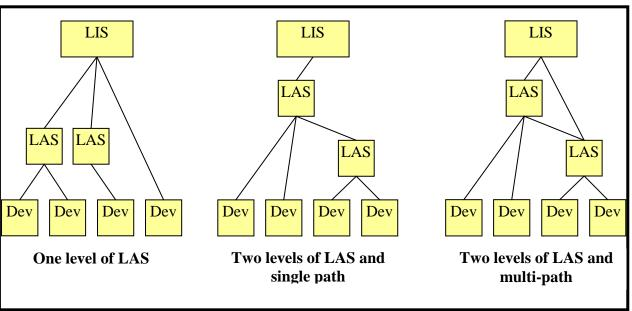
Figure 5.3-1: Systems interconnections in laboratory
