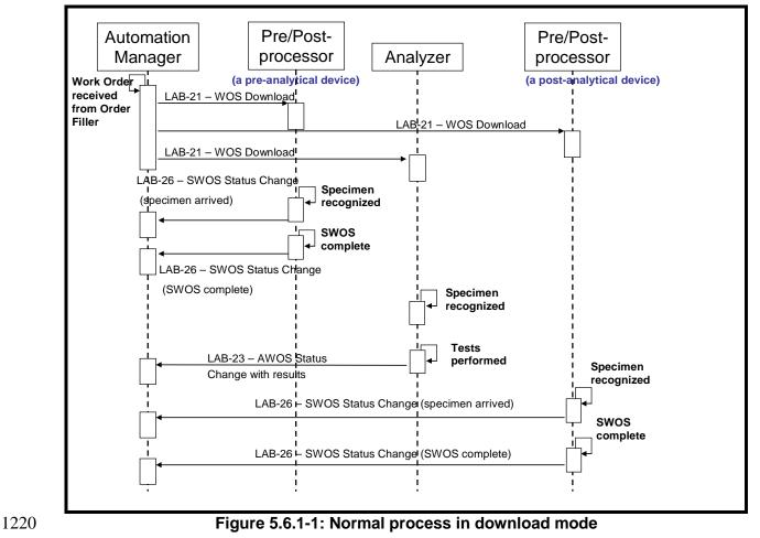
This diagram shows a situation with one pre-analytical device, one analyzer and one postanalytical device.
