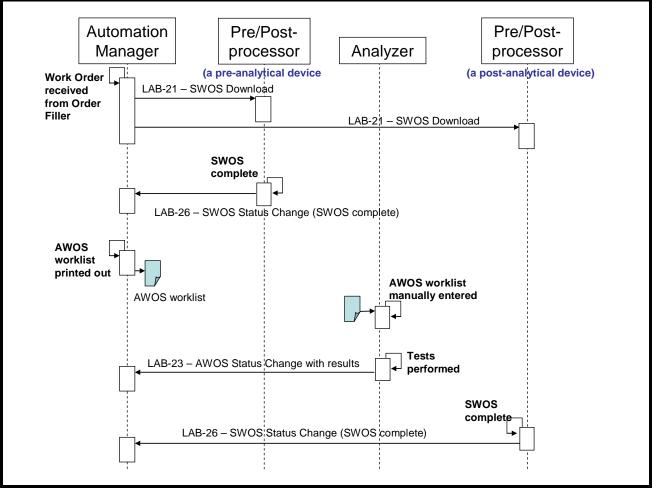
Figure 5.6.3-1: Normal process with AWOS manual entry
