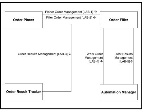
Figure 4.3-1: Laboratory Testing Workflow Actor Diagram
