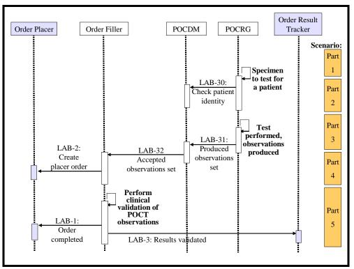
Figure 6.7.2-1: Process flow for use case 6.4.2
