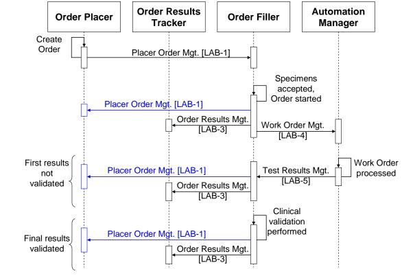
Figure 4.5.1-1: Process flow for placer ordering
