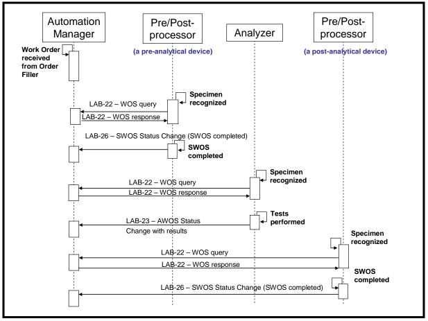
Figure 5.6.4-1: Normal process in query mode
