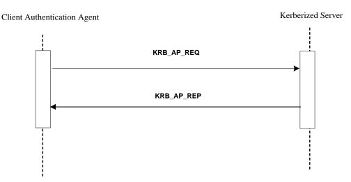
Figure 3.4-1: Kerberized Communications
