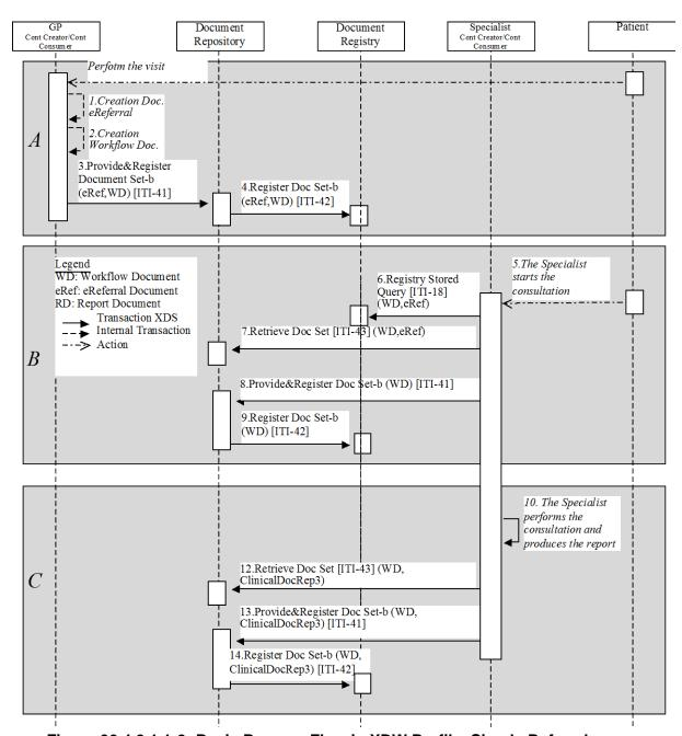
Figure 30.4.2.1.1-2: Basic Process Flow in XDW Profile, Simple Referral use case
