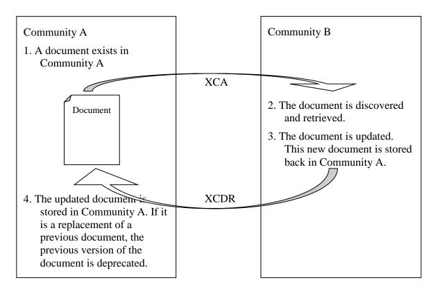
Figure 40.4.1-2: XCDR with XCA Example
