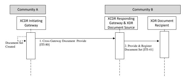
Figure 40.4.2.2.1: Remote Community with XDR Process Diagram
