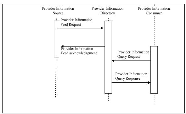
Figure 28.3.2.1-1: Basic Process Flow in HPD Profile
