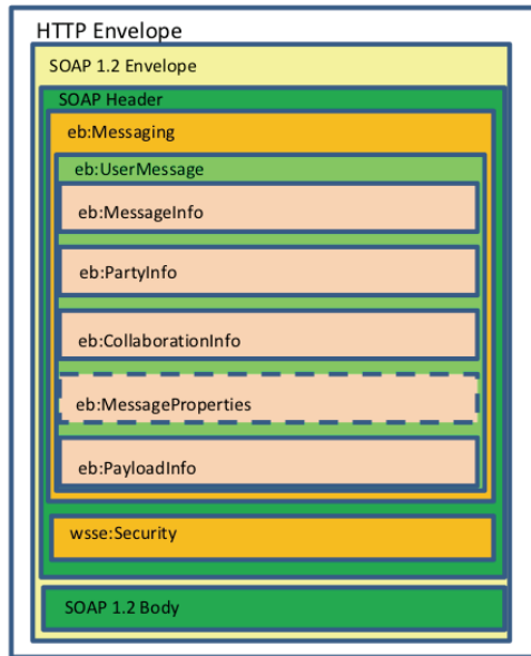
Figure V.4.4.2-1: Envelope with one single XML payload
