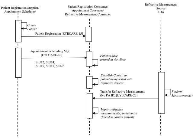
Figure 9.4.7-1: Refractive Measurements Model without Patient ID - Administrative Process Flow
