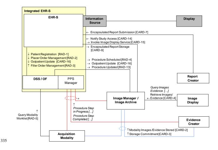
Figure 10.1-1. Image-Enabled Office Actor/Transaction Diagram
