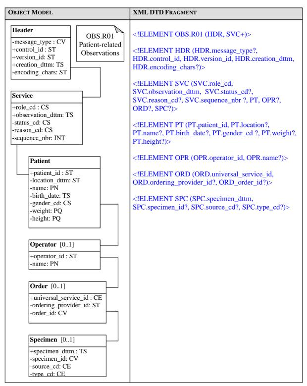
Figure 13-3: Message OBS.R01 in Transaction LAB-30
