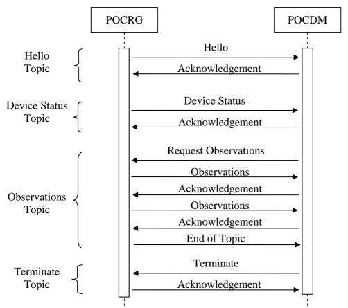
Figure B-2. Error-Free Basic Profile Flow, POCT1-A – Appendix B
