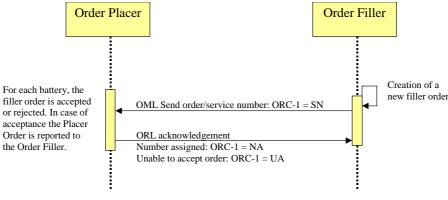
Figure 5.4-1: Process of a filler order
