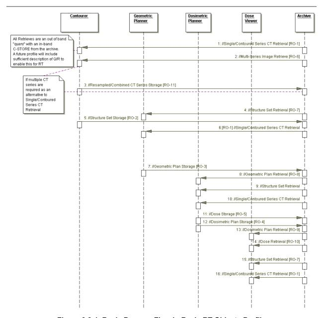
Figure 3.3-1. Basic Process Flow in Basic RT Objects Profile
