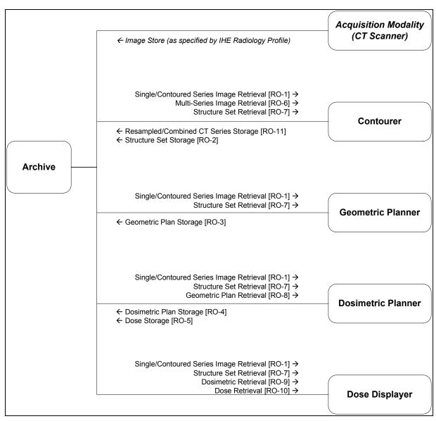
Figure 3.1-1. Basic RT Objects Actor Diagram
