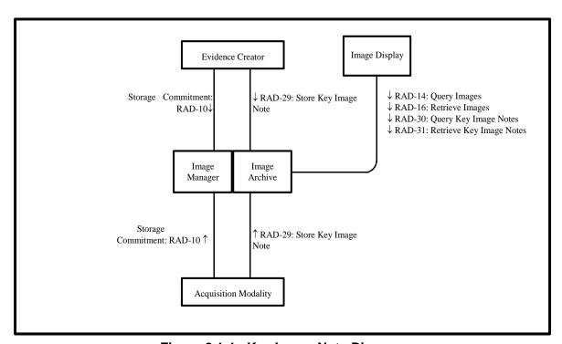
Figure 8.1-1. Key Image Note Diagram
