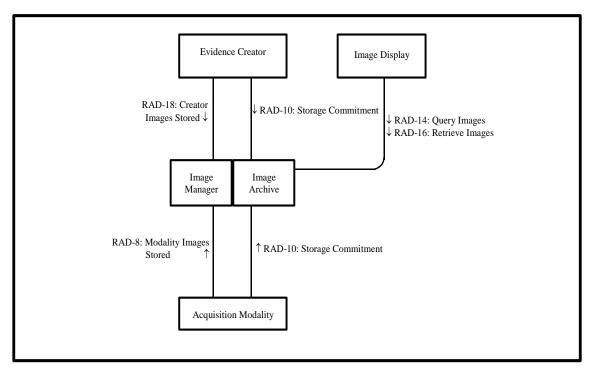
Figure 16.1-1. NM Image Actor Diagram
