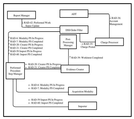
Figure 11.1-1. Charge Posting Transaction Diagram
