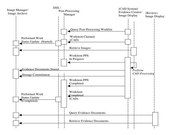
Figure 14.2-2. Evidence Document Management In Post-Processing Workflow
