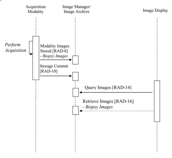
Figure 32.4.2.2-1: Basic Process Flow in SMI Profile
