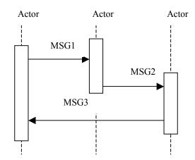
The interaction diagrams used in the IHE-PCD Technical Framework are modeled after those described in Grady Booch, James Rumbaugh, and Ivar Jacobson, The Unified Modeling Language User Guide, ISBN 0-201-57168-4. Simple acknowledgment messages are often omitted from the diagrams for brevity. One or more messages may be required to satisfy a transaction. Each message is represented as an arrow starting from the Actor initiating the message.
