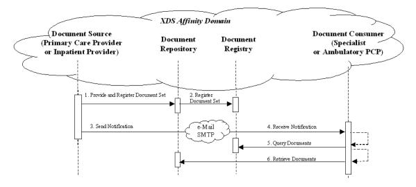
Figure 2.1-2 Use Case Process Flow Diagram
