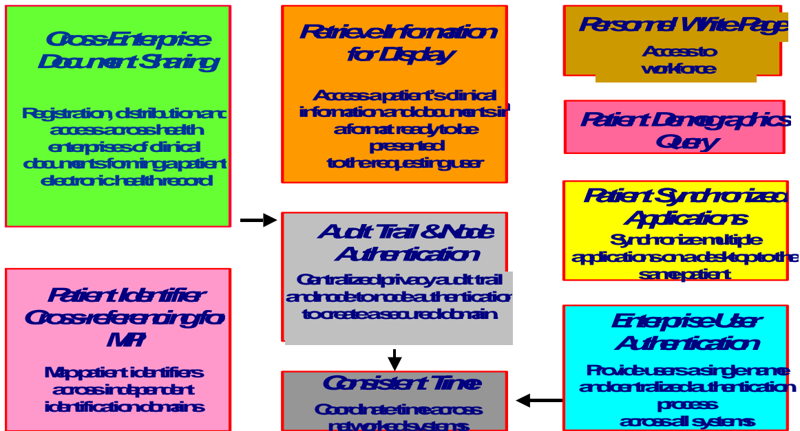
Figure 2-1 IHE IT Infrastructure Integration Profiles
