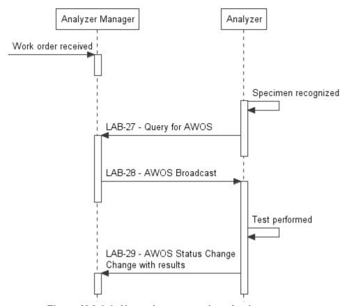
Figure X.6.1-1: Normal process when Analyzers query
