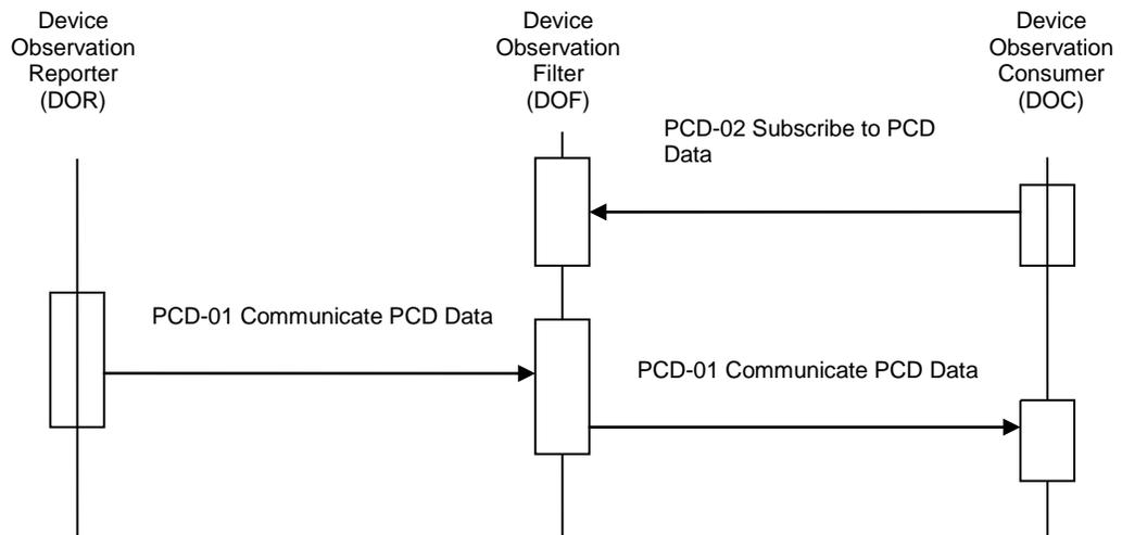
Figure 3.2.4-1 Subscribe to PCD Data Interaction Diagram
