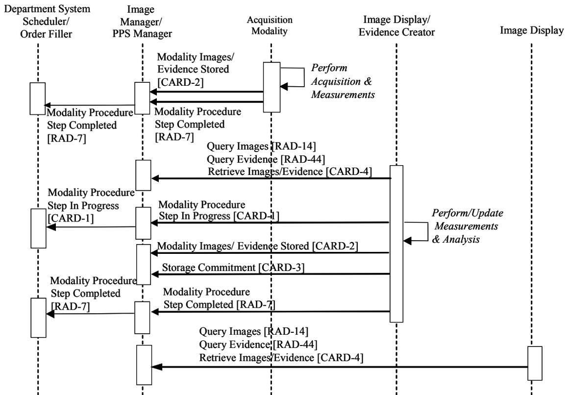
**Figure 4.3-6. Echo Measurement Evidence Creation– Case E7**
